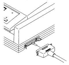
• Clip the cable into the socket using the wire clips on either side of the socket.
