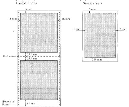
If you print outside these limits, you run the risk of damaging the printer mechanism (and tearing the paper or jamming it as it goes through the printer).
