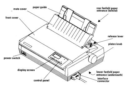
The printer (with interface cable connected)
