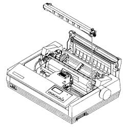
• Hold the roller unit so that the top is tilted slightly away from you. Slide the hooks on either side of the back of the roller unit over the platen (the large black roller) and under the silver bar behind and above the platen. The hooks should both be between the metal plates at either end of the silver bar.
