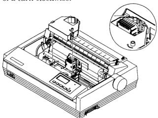
• Once the cartridge is in the carrier, tighten the ribbon again by turning the cartridge knob clockwise (about 1/2 a turn). Check once more to make sure that the ribbon is between the print head and print head shield (if it isn't, take the cartridge out, and try again).
