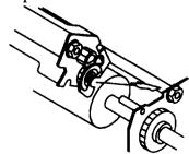
Push the front of the roller unit down firmly, so that the unit "clicks" into place. If it does not fit properly, remove it and try again.
