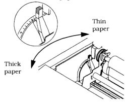
As you move the lever, you can feel it click between the six different positions. Position number 2 (starting from the rearmost position) is the one you will generally use for single sheets of paper (fanfold or cut sheet). Here is a table for the adjustment lever when you use multi-part sets.
