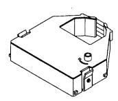
• Place the cartridge on the cartridge carrier inside the printer. Make sure that the ribbon is between the print head and the print head shield. Press the cartridge so that it "clicks" into place. If the cartridge does not "click" into position on both sides, you may need to turn the cartridge knob about 1/4 of a turn clockwise.
