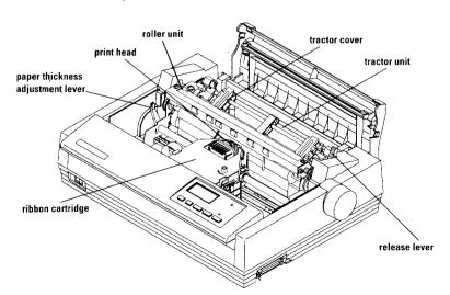
The printer with the front and rear covers removed and no interface cable connected
