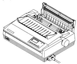
Open the tractor pin covers and align the holes in the fanfold paper with the pins on the tractor unit. You will probably need to slide the tractor pin units left and right to align the paper properly. Use the gray locking levers on each tractor pin unit to allow the unit to slide left and right along the rail. Remember to lock each tractor pin unit in place again when you have finished moving it.
