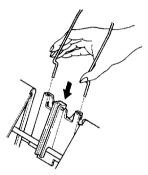
• Fit the stacker attachment into the fixing groove in the front of the sheet feeder. You may need to squeeze the stacker attachment a little to fit it.
