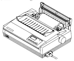
• Close the pin unit covers after you have made sure that the paper holes are properly lined up with the tractor pins. If the holes and pins are not correctly lined up, you may find that the paper tears and jams.
